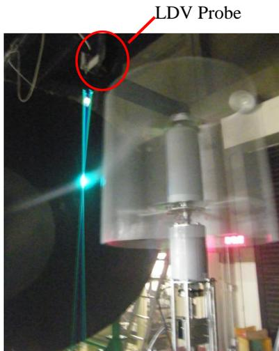
Fig. 5 LDV Measurement of VAWT Rotor
